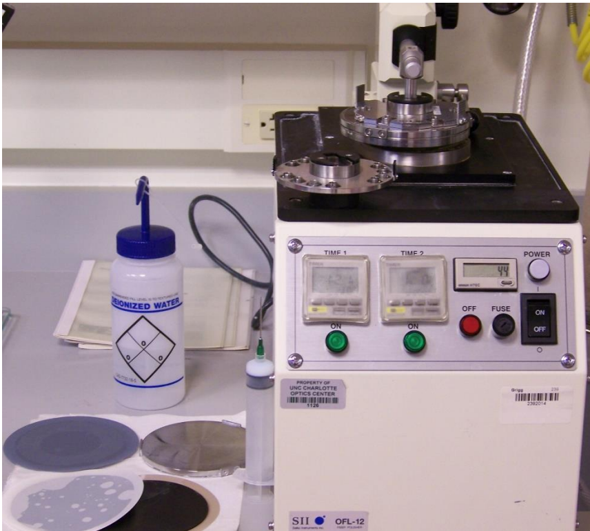
Seiko Instruments Optical Fiber Polishing Machine Model: OFL-12
