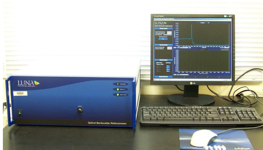
Luna Technologies Optical Backscatter Reflectometer Model: OBR
