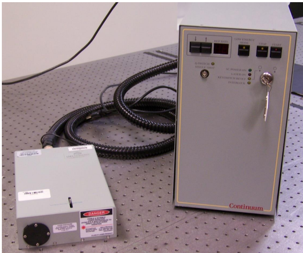
Continuum Nd:Yag Laser Model: MiniLite II
