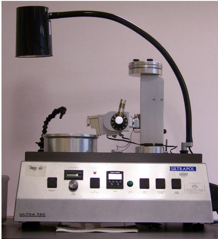
Ultra Tec Ultrapol Fiber Lens Polisher Model: 6380.1
